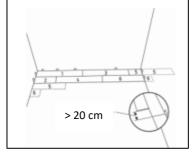
Always ensure that the ends of the tiles in two successive rows are the same and that the distance between the short ends is at least 20 cm.
