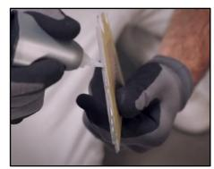
In case of a double pipe, drill a hole with the same diameter as the pipes at all the marked points, adding 15 mm. If the pipes are on the long side of the board, make a 45 degree cut from each hole to the side
