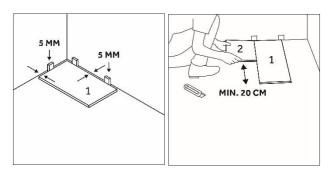
2. Now take a second tile and cut it to a minimum of 1/3 and a maximum of 2/3 of a panel length as a starting tile (n°2) for the second row.
